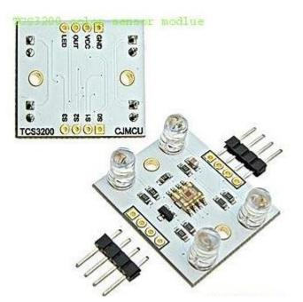
Color sensor TCS230 TCS3200D color module /identification module/ color sensing PCB Board(white)
