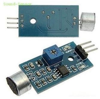
Sensitivity Control Potentiometer Sound Detection Sensor Module Sound Sensor car Features:
