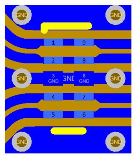
Figure 21. USB 3.1 Gen 2 SuperSpeed Layout
