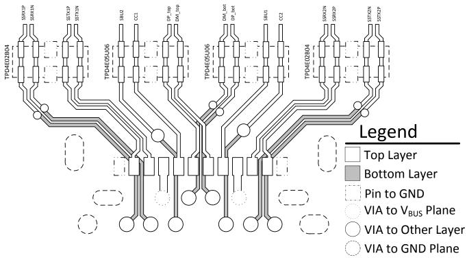
Figure 24. USB Type-C Mid-Mount, Hybrid Connector with One-Sided ESD Layout
