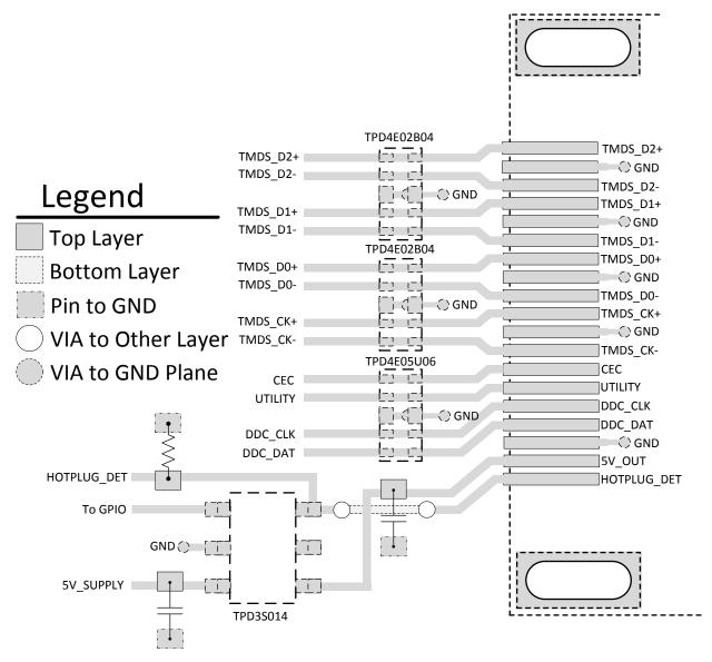
Figure 25. HDMI2.0 Type-A Transmitter Port Layout
